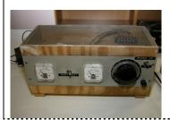
conservatively rated at 20 volts / 15 amps and uses a Variac (voltage divider-type) throttle for super smooth operation.
