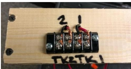
Back of module showing terminal block for hooking up power packs
